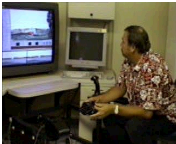
Figure 7: Pilot-in-the-loop realtime simulation using RIPTIDE
